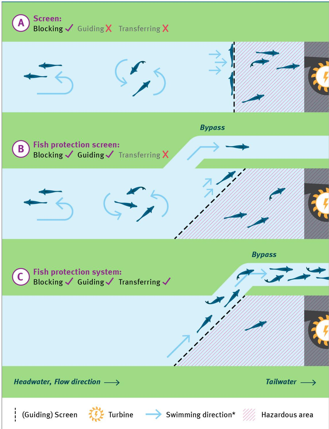
A fish protection system always consists of a fish protection screen and a bypass, designed as a functional unit.
